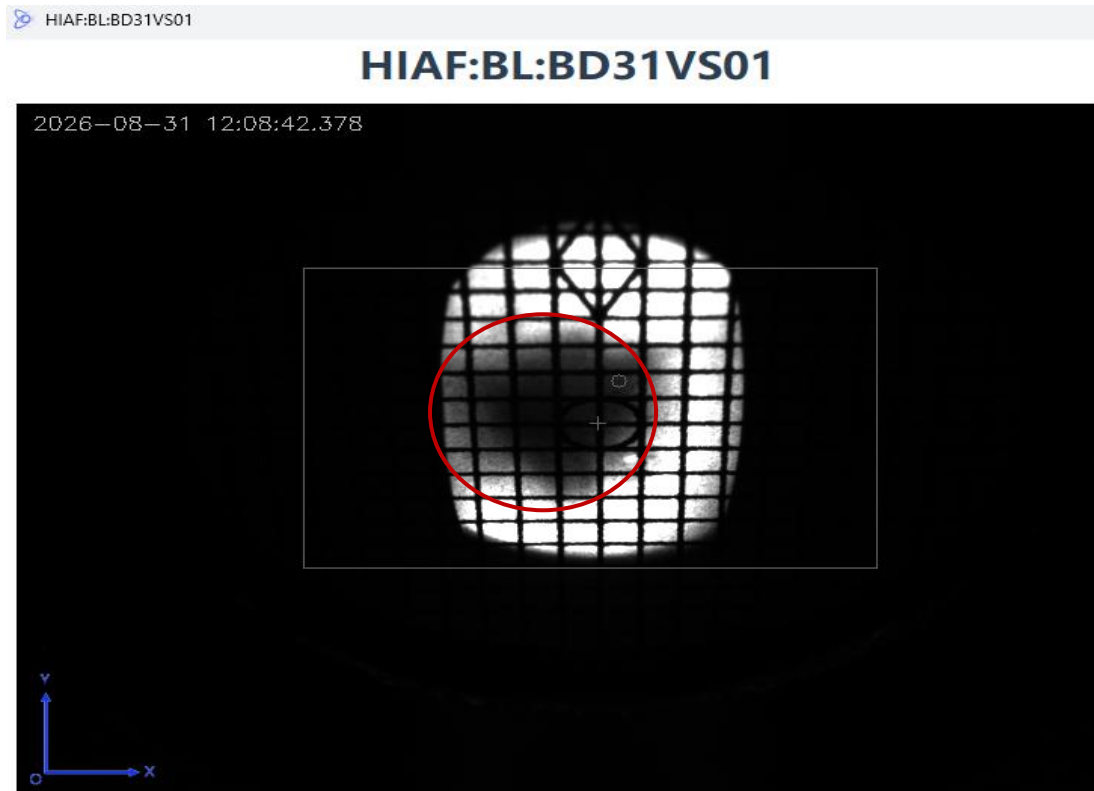
Coated powder VS darkening after a long-time beam shooting
